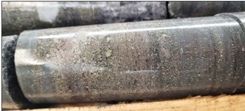
22.3 g/t Au | 0.7 m (254.3 m – 255.0 m) semi-massive "buckshot" pyrite with sphalerite and pyrrhotite
